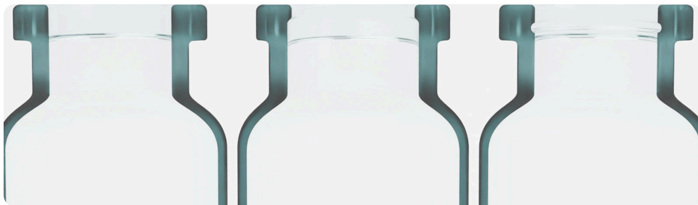
Sectioned 10R necks, left to right: no blowback, European blowback, American blowback.
