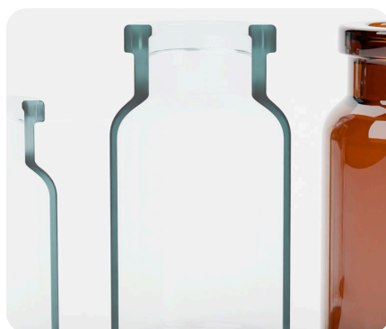
Sectioned 10R necks, left to right: no blowback, European blowback, American blowback.
