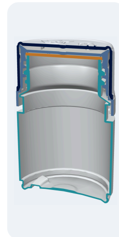
Engineering sections from PSI development work: CRC 38 closure, 60 ml bottle with closure, CRC 28 with moulded liner.
