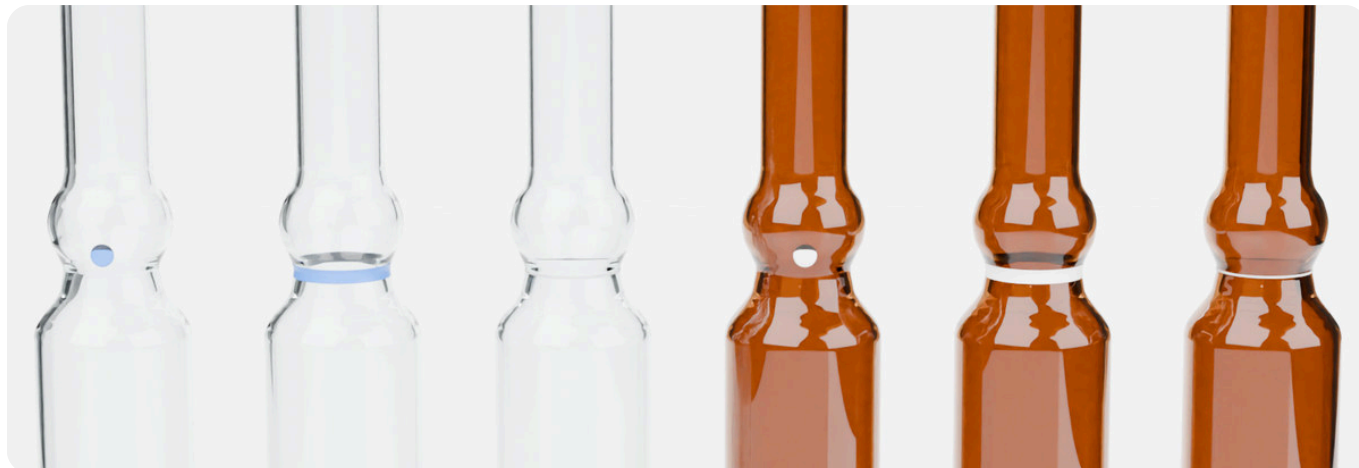
Break systems close-up: one-point-cut dot, colour break ring and score ring on clear and amber glass.
